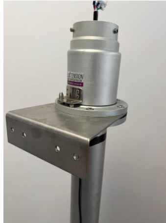
Correct mounting plate attachment
