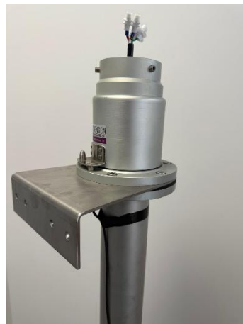
Correct mounting plate attachment
